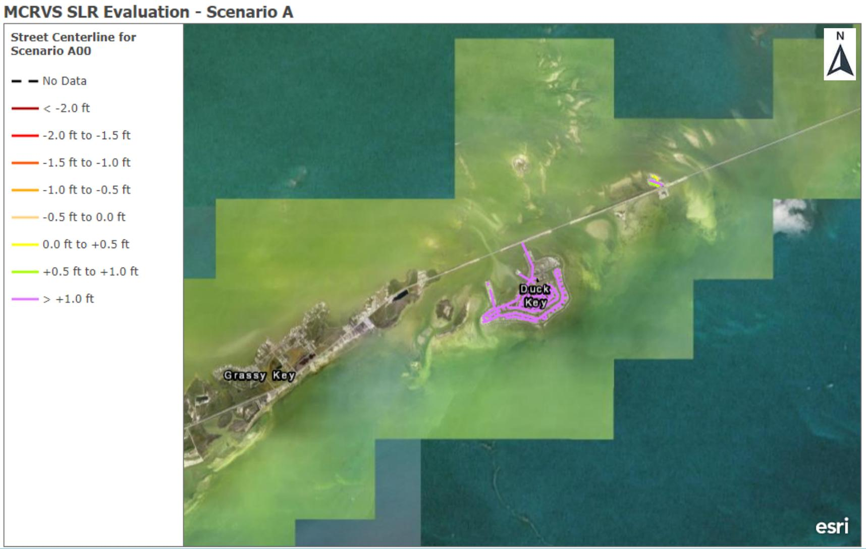
FIGURE 5. MIDDLE KEYS SCENARIO A00 – CLEARANCE BETWEEN ROAD ELEVATION AND MHHW
