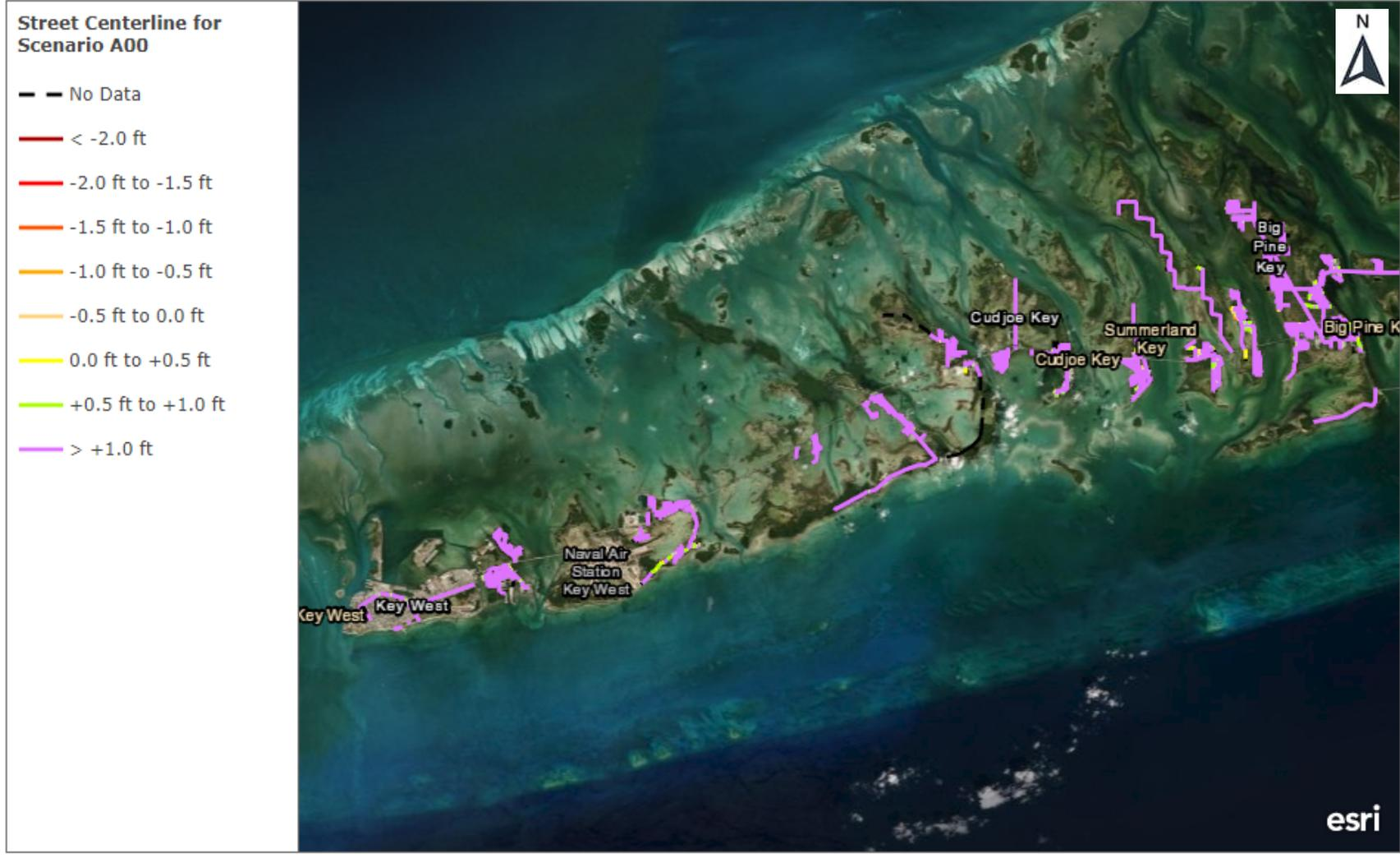
FIGURE 6. LOWER KEYS SCENCARIO A00 – CLEARANCE BETWEEN ROAD ELEVATION AND MHHW
